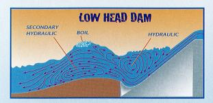
Even small dams with a shallow drop create a dangerous backwash. During periods of high water and heavy rain, backwash currents often become stronger, extending farther downstream. A small low-head dam that may have appeared harmless at very low water can become a monstrous death trap when the water level rises. Boaters must become familiar with a river's worst danger and know the waters they plan to visit.
